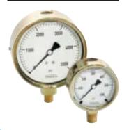
NOSHOK CAST BRASS CASE 300 SERIES GAUGES are the highest quality, most reliable liquid filled gauges available. Their one piece die cast brass case and heavy duty bourdon tube and movement enables them to stand up to shock and vibration encountered on the most demanding applications.
